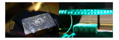
In collaboration with the RICH project and the ESAT labs, the **Royal Museums of Art and History** coordinates a pioneer project in which the multi-light Portable Light Dome is transformed into a Multi Spectral dome equipped with IR, Red, Green, Blue and UV LED light sources. This short video demonstrates the acquisition process with the fist developed MS microdome prototype of a Fayum mummy portrait (Egypt, Roman era) at the Brussels museum.
