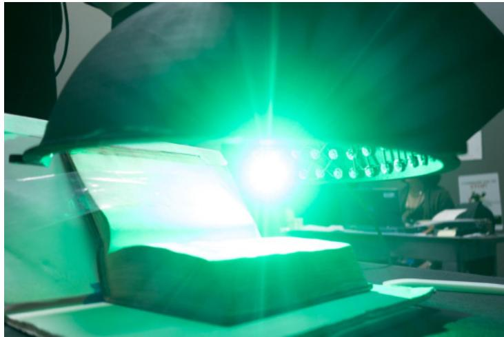
The tool is equipped with 228 different LED lamps. Five different spectra are evenly distributed over the dome: UV at 365 nm, Blue at 460 nm, Red at 523 nm, Green at 623 nm and IR at 850 nm. A black and white sensor of 28 Mp with extended sensitivity in UV and IR is mounted on top of the dome.
