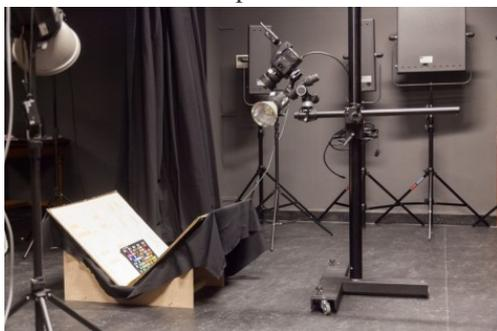
Photographing manuscripts closeby with high-resolution digital backs (80-100 million pixels) is also challenging as the tolerances you work within are very narrow. Depth of field, sharpness, vibration due to mirror slab, focus calibration, color calibration, diffraction, alignment, all come into play and can become problematic when not well controlled.
