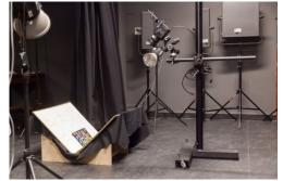
Photographing manuscripts closeby with high-resolution digital backs (80-100 million pixels) is also challenging as the tolerances you work within are very narrow. Depth of field, sharpness, vibration due to mirror slab, focus calibration, color calibration, diffraction, alignment, all come into play and can become problematic when not well controlled.
