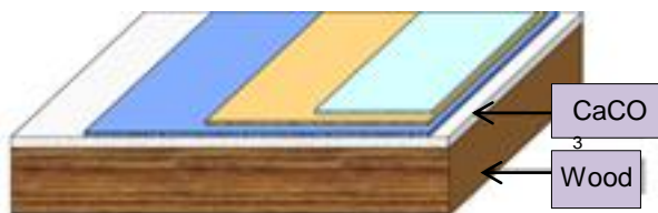
Fig. (up) Pigment panel, (down) Design of the 3d structure of the panel with combination of successive layers of pure pigments or of mixtures of them in each sub layer
