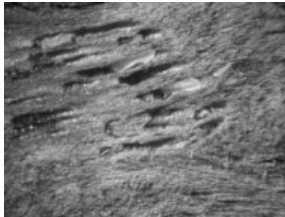
Figure 3.28. Initial shipworm infestation on pine and oak samples after 3 months.
