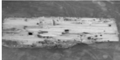
Figure 3.29. Archaeological oak and fresh pine samples degraded by shipworm after 12 months.
