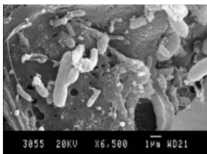
Figure 3.19. Presence of bacteria on pine and oak samples in anaerobic environment.
