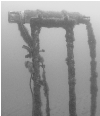
Figure 2: Data logger on Darss Cog site showing fouling.
